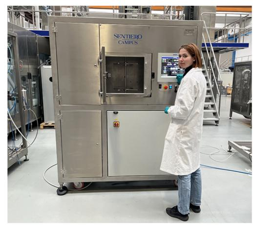
"We have developed a system that sterilizes personal protective equipment, allowing it to be reused instead of being discarded after initial use. Furthermore, as the protective device begins to deteriorate, our system enables it to be disposed of as recyclable waste, no longer categorized as special," explains Cecilia Muraro, Reliability Engineer at II Sentiero International Campus, who oversaw all stages of the research.
