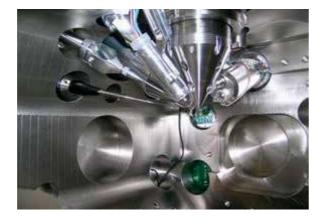
tion systems (GIS) for deposition of protective layers, and a Omniprobe micromanipulator which allows to pick up the lamella and to transfer it on the TEM grid always inside the chamber.
